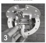
Screw the new mooring line into the "line attachment."
