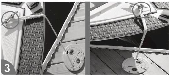
Whether using the EYE or the SNAP HOOK, simply attach the line to your boat.
